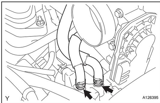
**5. REMOVE THROTTLE WITH MOTOR BODY ASSEMBLY**
