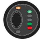
Main Fuel Tank – Automatic Shut Off Set while Fill Disabled
