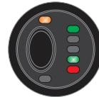
Once the options have been set wait for 10 seconds, the buzzer will sound with a double beep to indicate that the second part is complete. If both option are set the unit will exit the program mode and return to normal operation mode. Otherwise it will proceed to the third part of the program mode.
