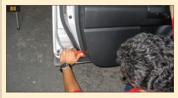
shield stand or workstation. Reach over, place your elbow on the setting pad and set the windshield on the urethane at the mark you made during dry fit. Lower the driver's side of the windshield onto the urethane and line it up with the dry-fit mark; it is now in place.
