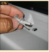
strip channel and not on the backside of the metal carrier. Align the carrier before bolting it to the plastic hardware on the glass.
